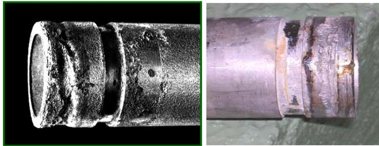
Figure 7. Crevice corrosion under Victualic couplings in high-pressure piping made of 316L (Jeddah-left) and 904L (Spain-right).
