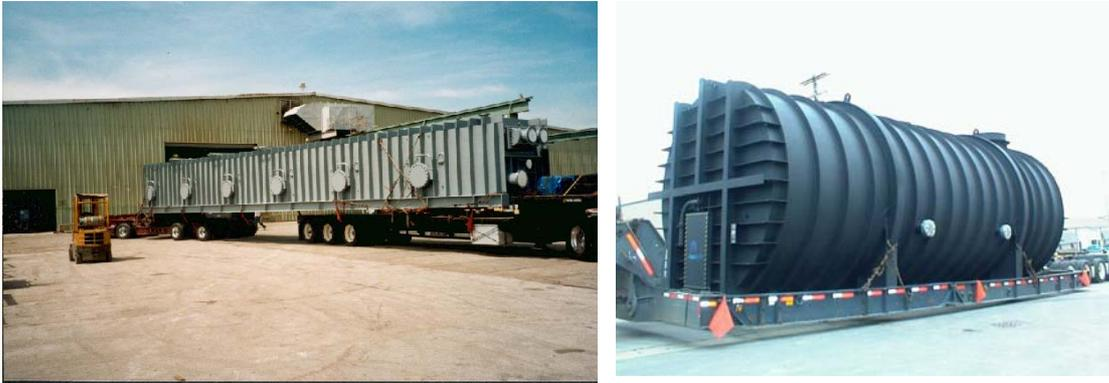
Figure 5. Evaporator shells made of solid 254 SMO for an MSF once-through plant (left) and an LT-MED plant (right).
