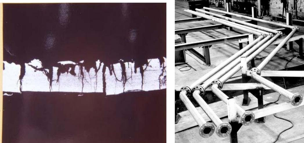
Figure 2. Severe bromide induced stress corrosion cracking of 316L in the vent system of Ras Abu Fontas (left) and the remedy, the installation of 904L drain legs (right).
